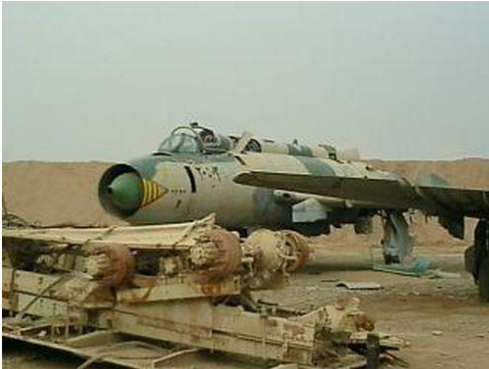
Some of IrAF aircraft - like this Su-20M - were found left in open, but already "cannibalized" for spares.
